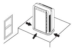
Do not place it near the window where the curtain may cover the Intake and out flow of the air.
