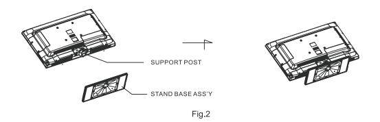
Step 3: then use the screwdriver to fix them together with screws
