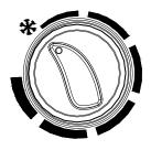
Set the thermostat to "max." and operate the appliance until the desired room temperature is reached. Turn the thermostat anticlockwise until the appliance switches off with an audible "click".
