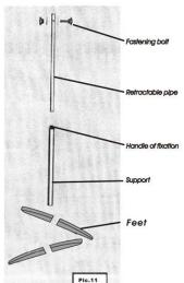
Installation of the heater on the telescopic prop is done by the help of the fastening bolt, by the figured screw-nut (Figure 11) and the brackets, which are fastened on the retractable pipe (Figure 11)
