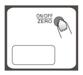
To maximize battery life, please press  $\frac{ON/OFF}{ZERO}$  button for 3 seconds to turn off scale after use.
