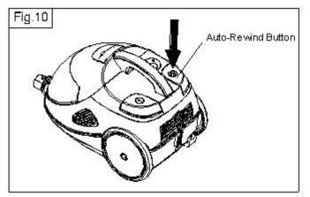
**Caution:** While nearing the end of the retraction, hold on to the end of the cord and guide it into the cord storage compartment. The force and speed of the retraction may cause the plug to snap back and hit something.
